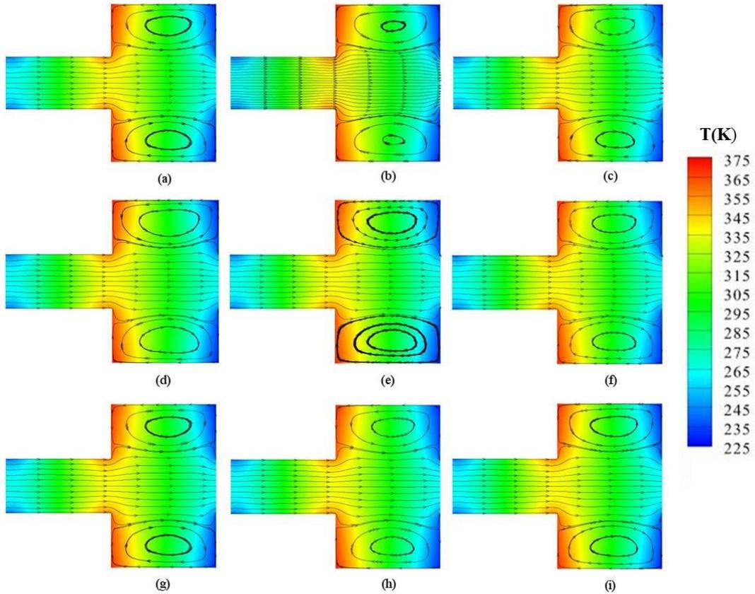
Figure 2: Streamlines and temperature contours for different gas compositions : (a)Ar; (b)N<sub>2</sub>; (c)O<sub>2</sub>; (d)N<sub>2</sub>&O<sub>2</sub>=4:1; (e)N<sub>2</sub>&O<sub>2</sub>=1:1; (f)N<sub>2</sub>&O<sub>2</sub>=1:4 and different molecular models: (g)HS model; (h)VHS model; (i)VSS model corresponding to case 1.
