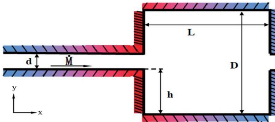
Figure 1: Knudsen pump in rectangular channel model
