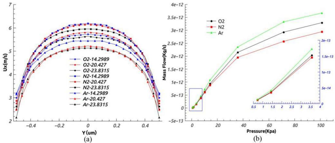
Figure 3: Under different pressures(14.2989,20.427,23.8315), (a)velocity  $U_x$  of three different gases for the reference case at  $X=1$ . (b) mass flow for three different gas at different pressures.
