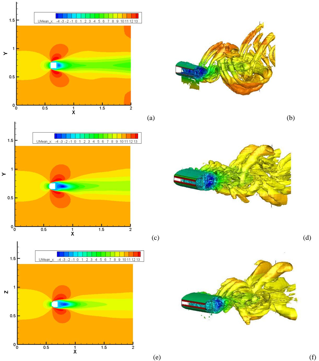
**Figure 3: Results of the mean velocity ( $U_x$ ) and the iso-surface of the second invariant of the velocity gradient ( $Q=100$ ) for different cases: (a)  $U_x$  for case F0; (b)  $Q$  for case F0; (c)  $U_x$  for case F1; (d)  $Q$  for case F1; (e)  $U_x$  for case F2; (f)  $Q$  for case F2.**
