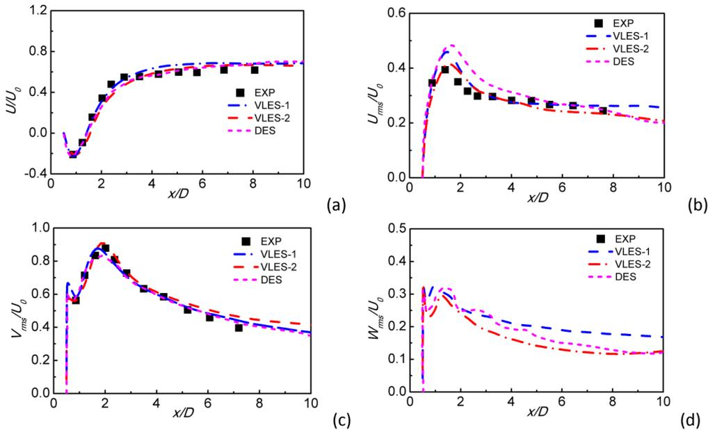
**Figure 2: Comparisons of mean and RMS velocities along the central line in the middle plane of the square cylinder. (a) mean velocity in the x direction; (b) RMS velocity in the x direction; (c) RMS velocity in the y direction and (d) RMS velocity in the z direction. Experimental data is from ref. [2] and DES results from ref. [9].**
