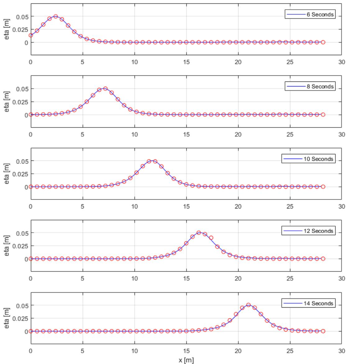
**Figure 1: Surface elevation for solitary wave propagation over a flat bottom. Dots represent the results of a SWASH standalone simulation over the complete domain. The blue line represents the results of the coupled model ( $0\text{ m} \leq x \leq 18\text{ m}$ : SWASH,  $18\text{ m} \leq x \leq 28\text{ m}$ : OpenFOAM).**
