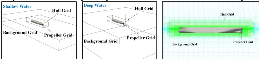
**Figure 1 The overset grid arrangement and the local grid distribution**
