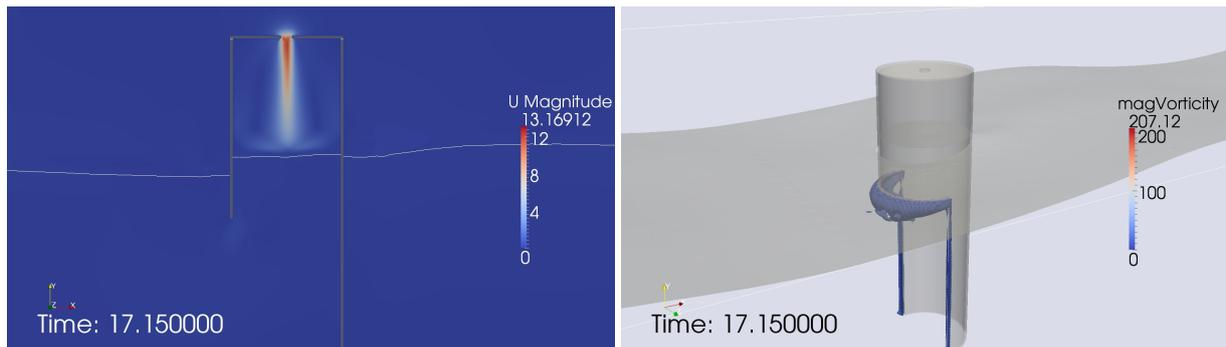
**Figure 4:** Left: an example of the simulated air velocity and the air-water interface. Right: An example of the simulated vorticity. For both panels,  $T = 1.0$  s,  $H = 0.04$  m, and  $h = 0.31$  m.
