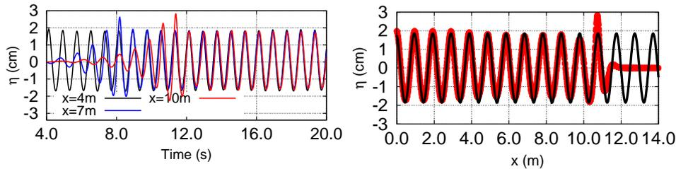
**Figure 2: Left: Times series of the waves measured at three locations in the numerical wave tank with  $x$  being the distance from the left end of the numerical wave tank. Right: A snapshot of the waves in the numerical wave tank with red line being the simulation result and the black line being the theoretical Airy wave solution.**
