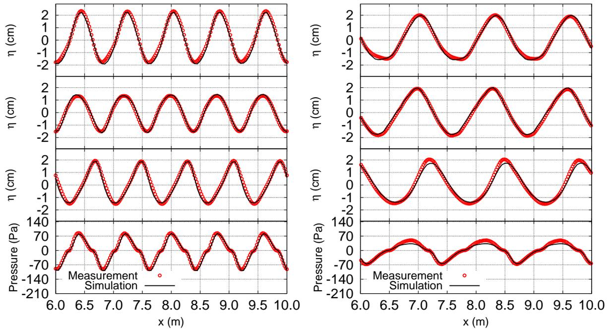
**Figure 3:** Comparisons between the simulated and measured surface displacements at three locations and the air pressure for  $T = 0.8$  s (left) and  $T = 1.3$  s (right). From top to bottom, the plots show the measured surface displacements at the locations  $G_1$ ,  $G_2$  and  $G_3$ , and the relative air pressure. The circles are measurement and the solid lines are numerical simulations.
