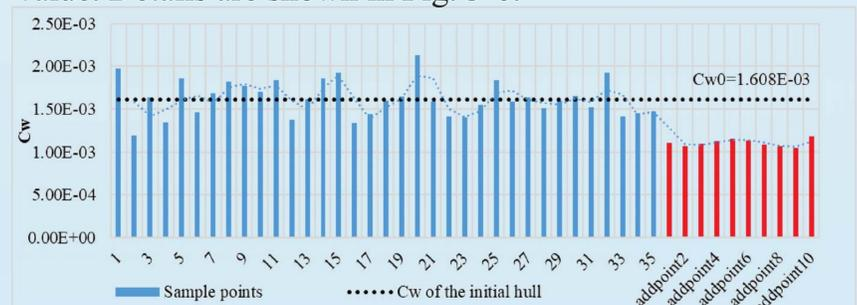
Figure 3: The initial sample hulls and the additional new hulls used in the EGO method
