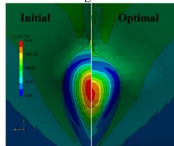
**Figure 8: Contour plot of the pressure distribution of the initial and the optimal hull forms (Fr=0.26)**
