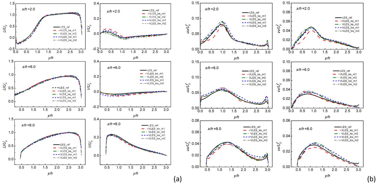
Figure 4: Comparisons of the mean velocities (left) and Reynolds stresses by the present VLES modelling with reference LES results [9] in the periodic hill flow, at different downstream locations.
