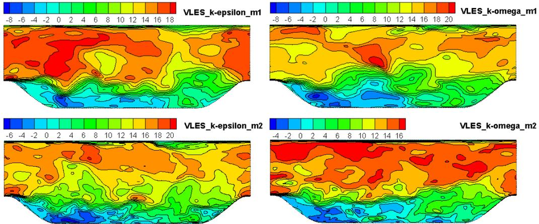
Figure 3: Instantaneous velocity distributions for periodic hill flow with different VLES modelling.
