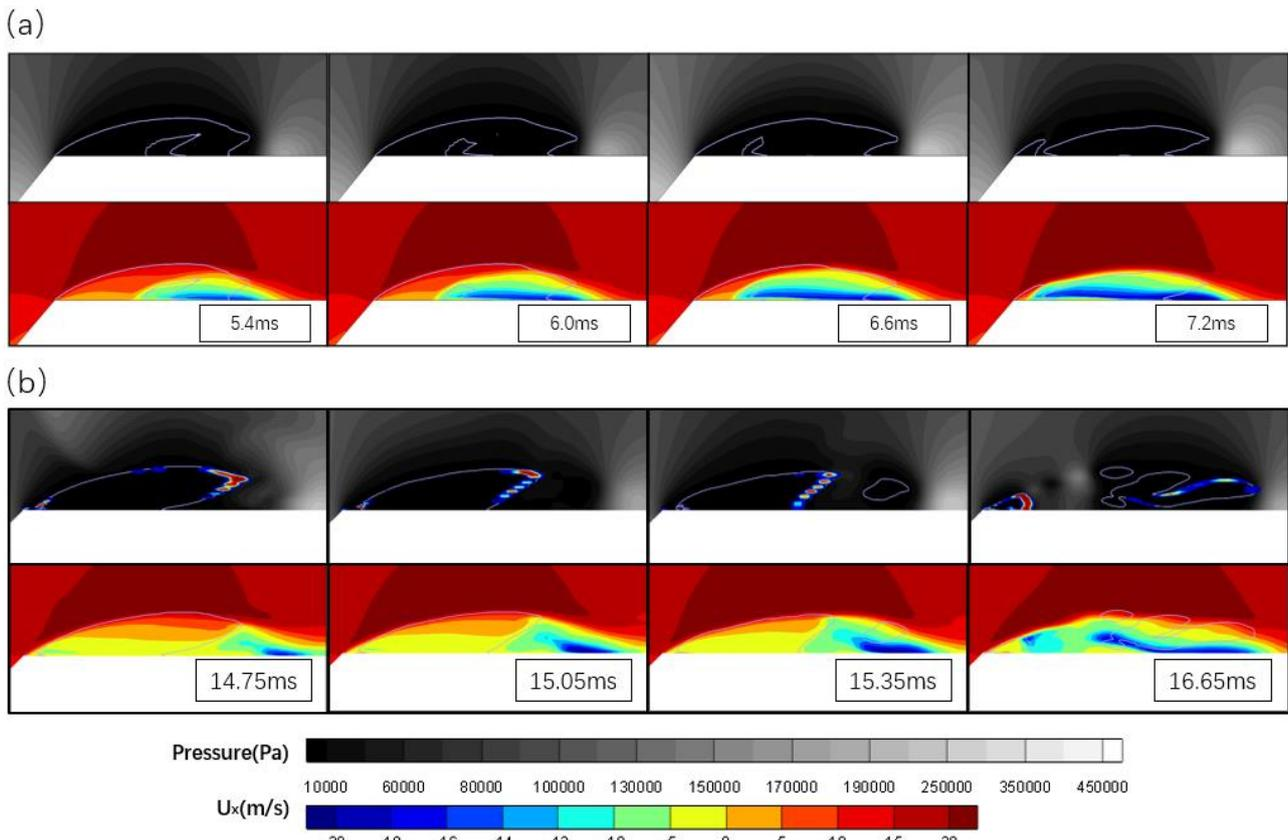
**Figure 3: Pressure fields with condensation rate and velocity fields: (a)the first half cycle, (b)the last half cycle**
