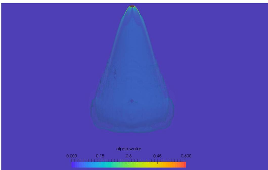
**Figure 1. Water sprinkler modelled with uncoupled Eulerian spray.**
