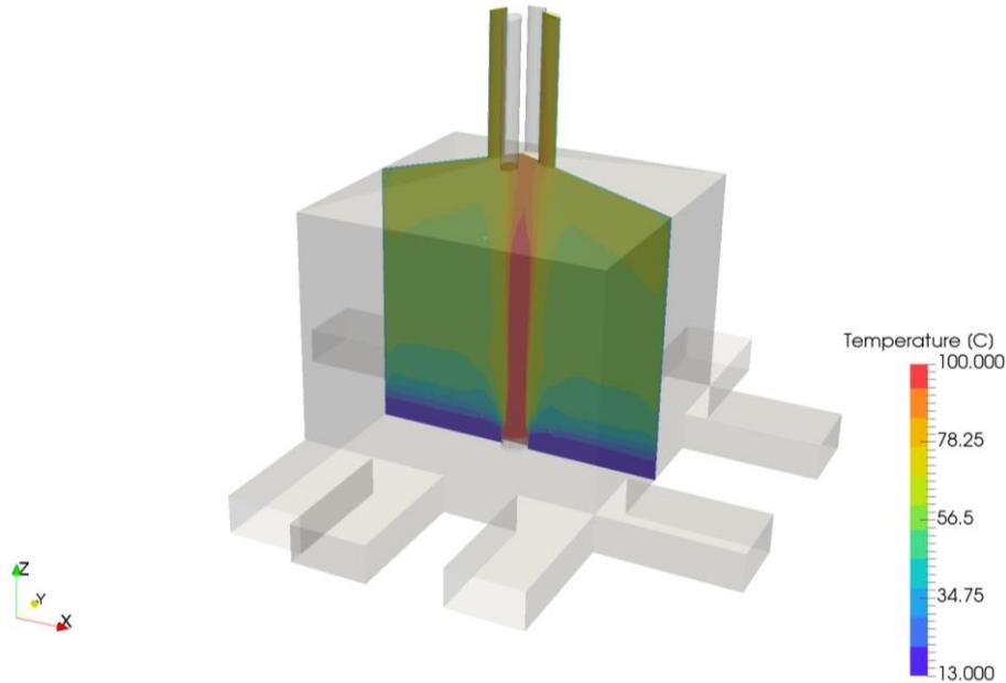
**Figure 2 Temperature plume developed for the Murcia facility case**
