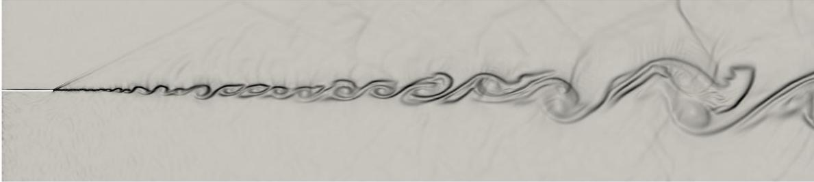
(b) Numerical schlieren contour of Case 2.
