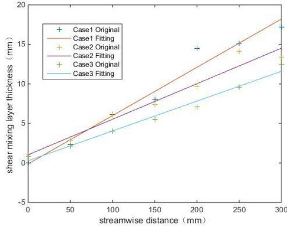
Figure 4: Thickness of shear mixing layer of Case1-Case3.
