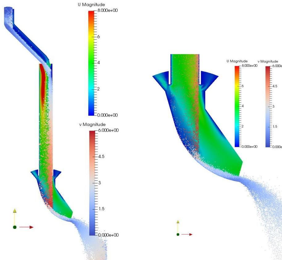
Figure 4: gas phase and particle phase velocity ( U-gas velocity; V-phase velocity)
