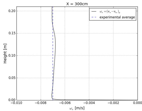
**Figure 3: Comparison of the numerical profile of sediment fall velocity as calculated using the two-way coupled approach, to the average of the experimental fall velocity at the X = 300 cm measurement station.**
