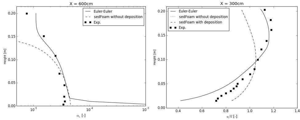
**Figure 2: Comparison of the numerical profiles of sediment volume fraction (left) and non-dimensional water velocity (right), of the two-way coupled approach (Euler-Euler) numerical profiles to the one-way coupled approach numerical profiles (sedFoam), and the experimental measurement at the X = 600cm and X = 300cm measurement stations.**
