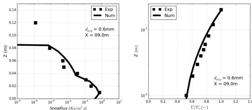
**Figure 1:** Comparison of the two-way coupled approach numerical profiles of snowflux (left) and non-dimensional airflow velocity (right), to the experimental measurement at the  $X = 9m$  measurement station, for an average particle size of  $0.6mm$ .
