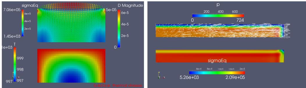
Figure 1: Combined FSI model for cases of thermal expansion of a solid brick and bar.
