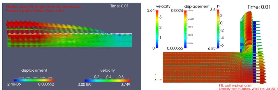
Figure 2: Conventional FSI cases: wave propagation in an elastic pipe and a jet impacting an elastic membrane.
