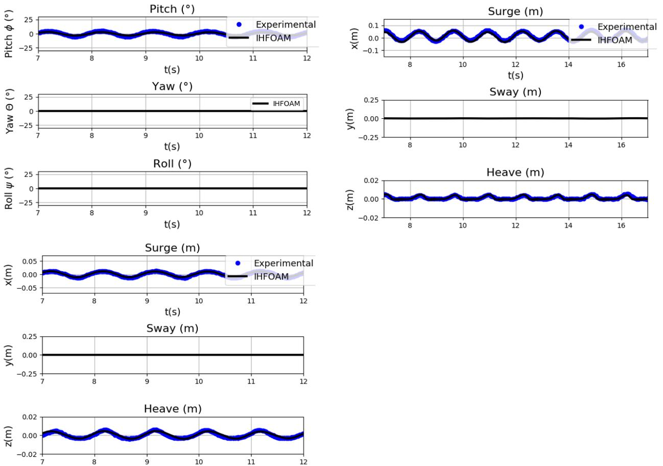
Figure 2: On the top: Case B:  $H = 3.1\text{cm}$ ,  $T = 1\text{s}$ ,  $h = 65\text{cm}$ . Pitch, Yaw and Roll (degrees) and Surge, Sway and Heave (m). On the bottom: Case A:  $H = 7.3\text{cm}$ ,  $T = 1.3\text{s}$ ,  $h = 65\text{cm}$ . Surge, Sway and Heave (m).
