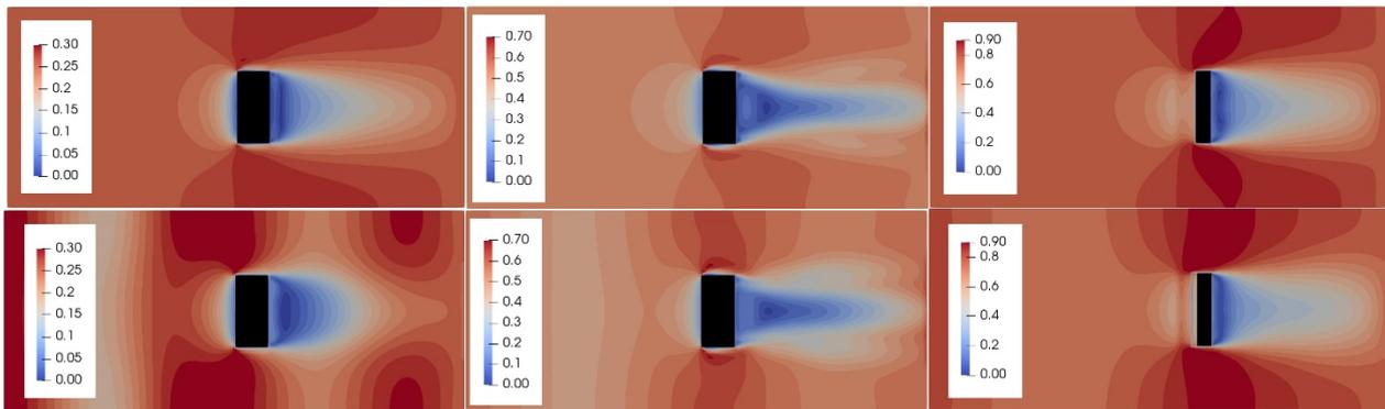
**Figure 4:** On the top, from the left to the right: velocity field magnitude  $U(\text{m/s})$  induced by only current of 0.25–0.5–0.75 m/s, respectively. On the bottom, from the left to the right: wave-current interaction with current intensities of 0.25–0.5–0.75 m/s, respectively. The wave case considered is: Case A:  $H = 7.3\text{cm}$ ,  $T = 1.3\text{s}$ ,  $h = 65\text{cm}$ .
