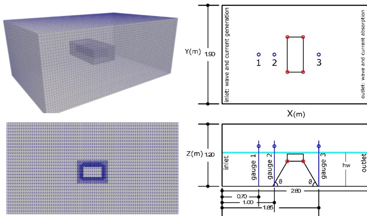
Figure 1: On the left: the global 3D mesh. On the bottom: a section of the mesh showing the two system of grids used to perform the overset mesh. On the right: Numerical wave tank developed.
