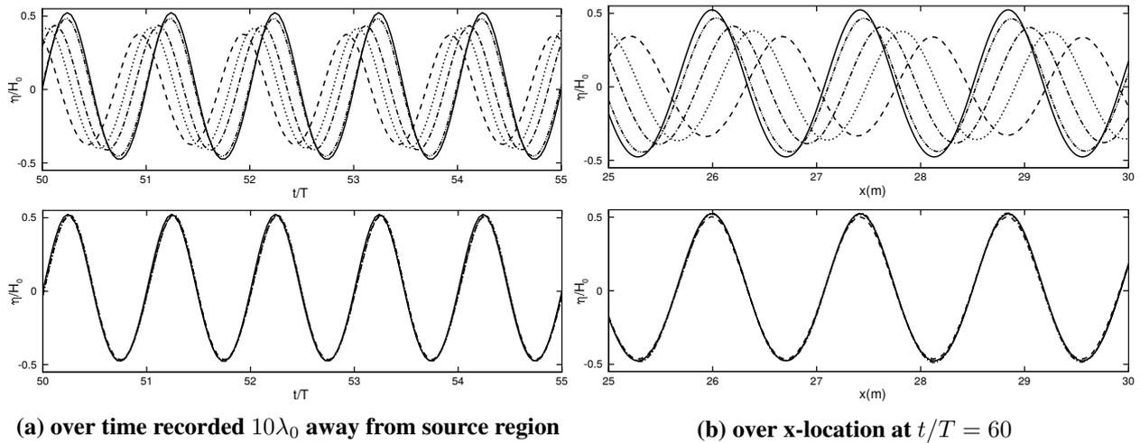
**Figure 3: Surface elevations for different time steps:** —,  $2^{nd}$ -order Stokes theory; ---, 0.008s; ·····, 0.004s; -·-·-, 0.002s; —·—·, 0.0002s, with interFoam solver(top) and the present solver(bottom)
