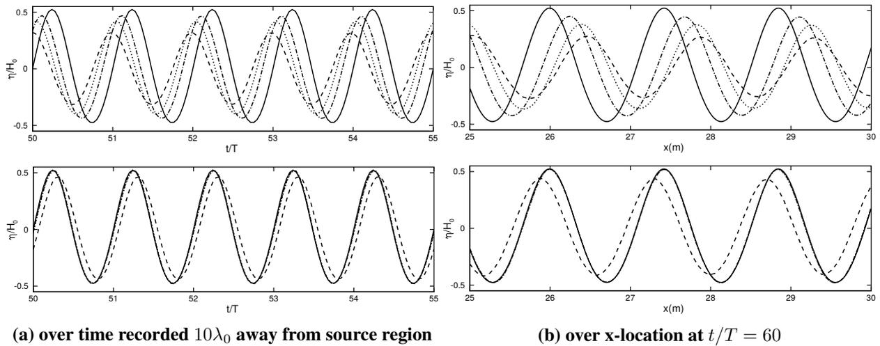
**Figure 4: Surface elevations for different grid resolutions:** —,  $2^{nd}$ -order Stokes theory; ---, 2 times coarser grid; ·····, reference grid; -·-·-, 2 times finer grid, with interFoam solver(top) and the present solver(bottom).
